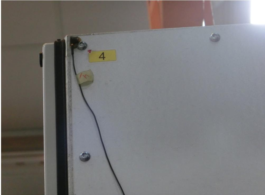
Photo 5 Measuring point A4: Upper right front corner of cabinet (Y-axis shown).
