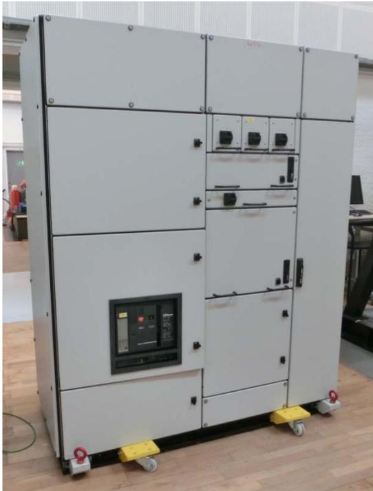
**Figure 1** Test object with initial door locking means (door at large circuit breaker not closed on this photo).
