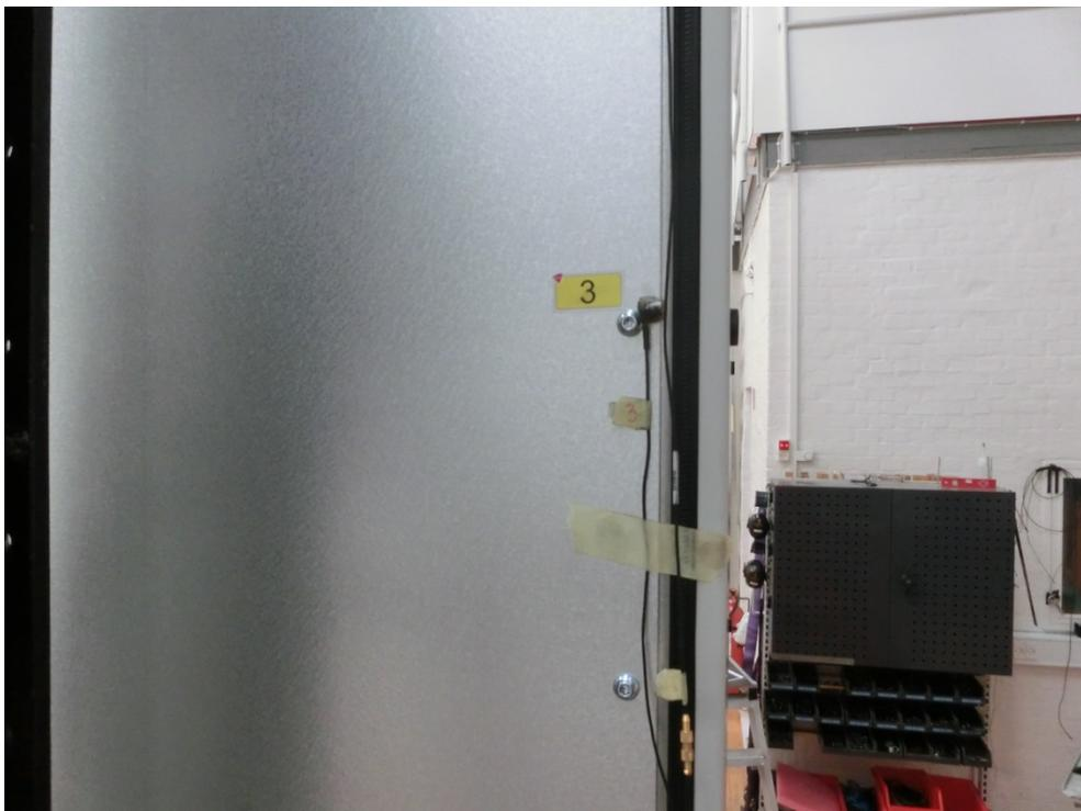
Photo 4 Measuring point A3: Middle of left front edge of cabinet (Y-axis shown).
