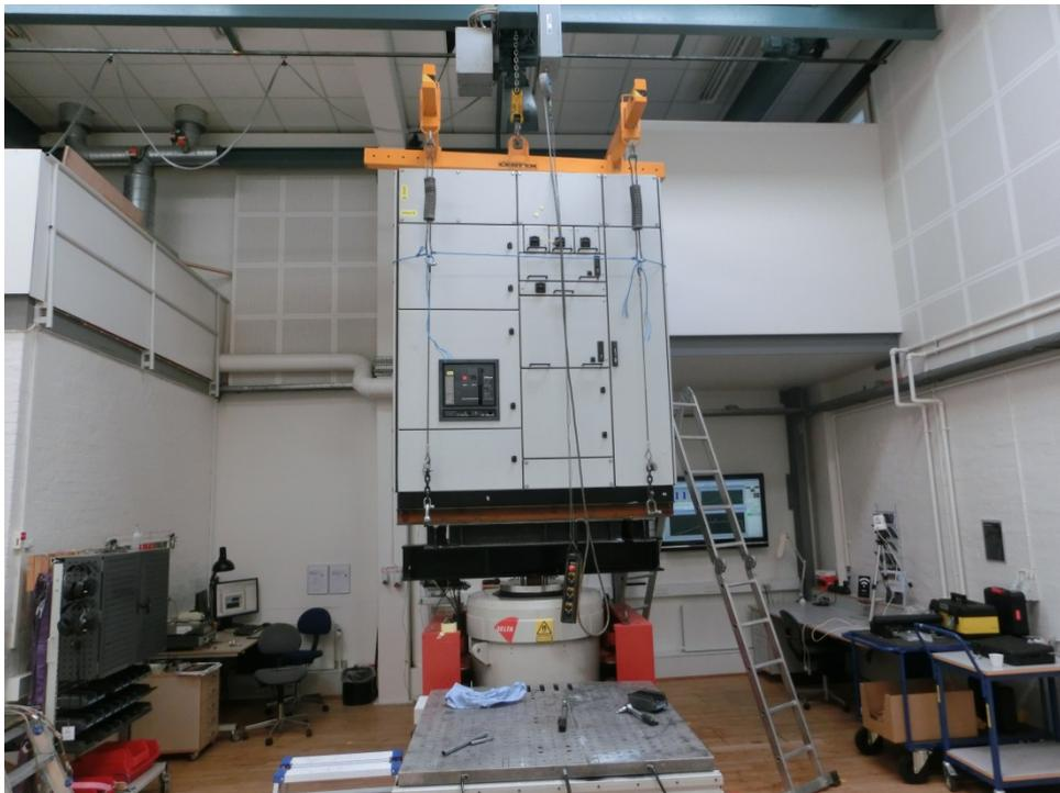
Photo 6 Test setup for Z-axis (note that the steel wires are used for carrying some of the weight via the fixture and are not attached to/supporting the test object).
