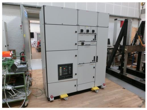
Photo 1 Test object before test (door at large circuit breaker not closed on this photo).
