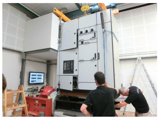
Photo 9 Visual Inspection after Y-axis: 2 front doors opened during exposure.
