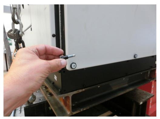
Photo 14 Visual Inspection: One mounting screw for right side plate fallen out.
