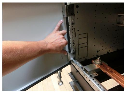
Photo 10 Visual Inspection after Y-axis: 2 front doors hinges loose.
