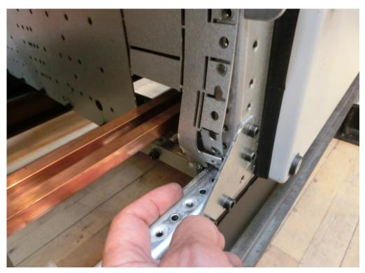
Photo 16 Visual Inspection: Buckling of lower right intermediate plate at front (near earth cupper bars).
