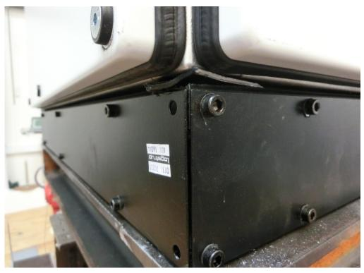
Photo 13 Visual Inspection: Black bottom frame broken at left side.
