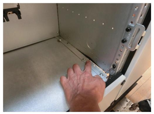
Photo 24 Visual Inspection: Buckling of lower cassette right side plate.
