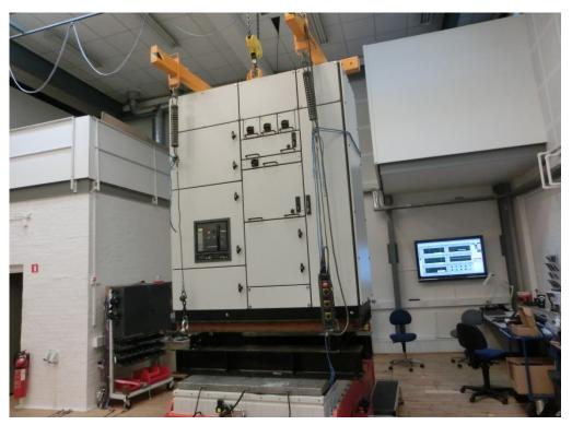
Photo 8 Test setup for X-axis.
