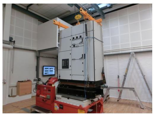
Photo 7 Test setup for Y-axis.
