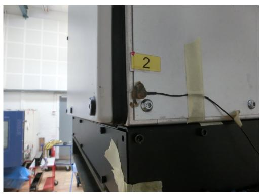
Photo 3 Measuring point A2: Lower right back corner of cabinet (Z-axis shown).
