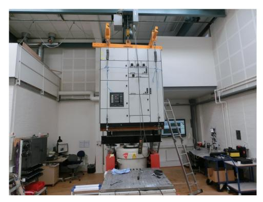
Photo 6 Test setup for Z-axis (note that the steel wires are used for carrying some of the weight via the fixture and are not attached to/supporting the test object.
