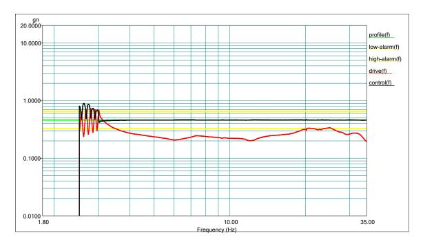
Curve 1 Recorded test level, Z-axis, black curve (the red curve is an internal vibration control channel).
