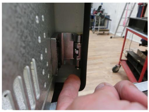
Photo 11 Visual Inspection after Y-axis: One hinge partly defect (lower "pin" fallen partly out).
